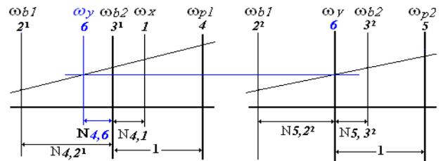
Figure 14. System nomograph for the Simpson gear train shown in Figure 13(a)
