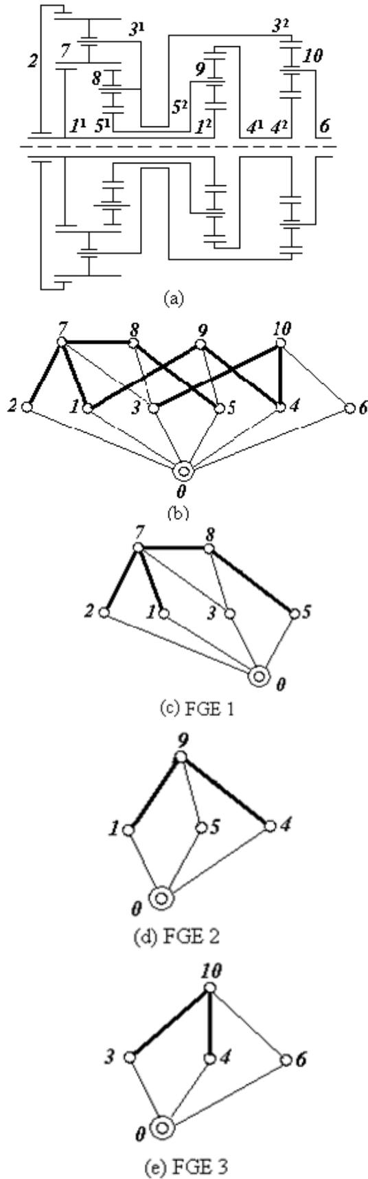
Figure 19. (a) schematic diagram, (b) canonical graph, (c) through (e) FGEs of a compound EGM.
