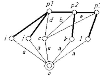
Figure 10. Graph of an FGE having three planets in a chain.
