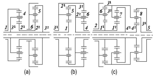
Figure 13. Some commonly used compound epicyclic gear trains. (a)Simpson gear train (b)Type-6206 gear train (c) Type-8001gear train
