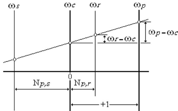
Figure 3. Nomograph for the basic epicyclic gear train.
