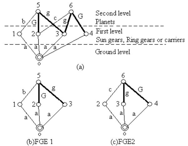
Figure 4. Canonical graph and FGEs of the mechanism in Figure 1
