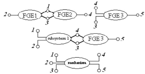
Figure 16. The unification process for type-8001 gear train
