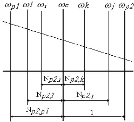
Figure 9. Nomograph for the double-planet FGT shown in Figure 7, in terms of the planet gear  $p_2$ .
