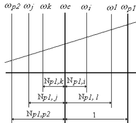
Figure 8. Nomograph for the double-planet FGT shown in Figure 7, in terms of the planet gear  $p1$
