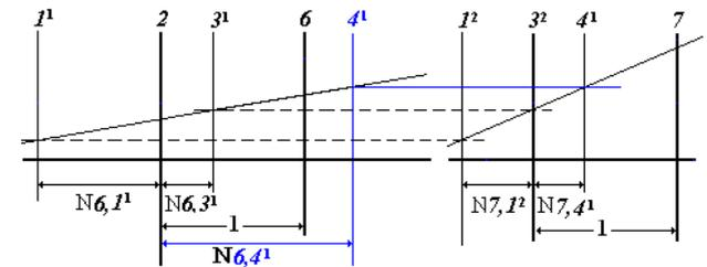
Figure 17. Nomographs for the first and second FGEs of type-8001 gear train and their unified subsystem.
