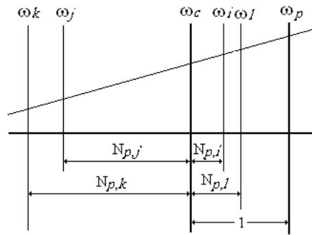
Figure 6. Nomograph for the single-planet FGT shown in Figure 5
