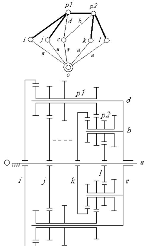
Figure 7. A typical double-planet FGT
